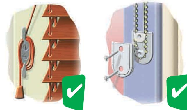
You can cut the dangerous loop out of some cords/chains and attach a tassel to the end of each strand. Some blinds will not operate without the loop, so get specialist advice before doing this.
